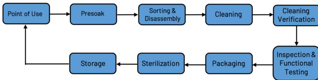
Figure 1: Reprocessing procedure flow chart
