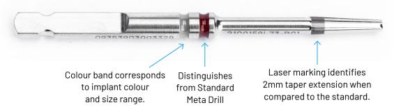
TIP: If using the extended metaphyseal drill, it is recommended to sink the drill head to the bottom of the black laser marking band ensuring it is still visible. This will provide a tight interference fit and assist in alleviating head forces.
