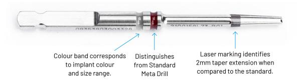
TIP: If using the extended metaphyseal drill, it is recommended to sink the drill head to the bottom of the black laser marking band ensuring it is still visible. This will provide a tight interference fit and assist in alleviating head forces.
